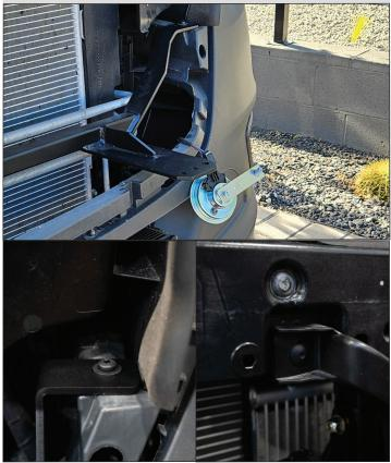
USING A 13MM SOCKET, TEMPORARILY REMOVE THE HORN. WITH THE HORN OUT OF THE WAY, GENTLY WORK THE GRILLE MOUNT INTO POSITION BY PULLING THE VERTICAL SUPPORT FORWARD TO MAKE ROOM TO ALIGN THE MOUNTING HOLE. SECURELY FASTEN THE GRILLE MOUNT USING THE OEM (2) T30 AND (2) T25 TORX HARDWARE FROM STEPS 2 & 3.
