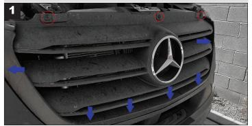
WITH THE HOOD OPEN. REMOVE THE (3) T25 SCREWS ALONG TOP FACE OF GRILLE SHROUD. THE ARROWS ON DIAGRAM INDICATE THE LOCATION OF (6) GRILLE TABS. WORKING FROM ONE SIDE OF THE VEHICLE TO THE OTHER, USE A PANEL REMOVAL TOOL TO DEPRESS THE GRILLE-TABS WHILE PULLING GRILLE FORWARD.
