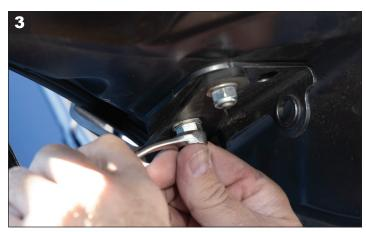
USING THE SUPPLIED WASHER AND NYLOCK NUT, SECURELY FASTEN THE DITCH MOUNTS TO THE HINGE.
