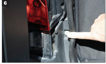
CONTINUE TO ROUTE THE WIRE EXTENSION DOWN THE REAR DRIVER-SIDE DOOR SEAL, USING THE PROVIDE ADHESIVE ZIP-TIE ANCHORS.
