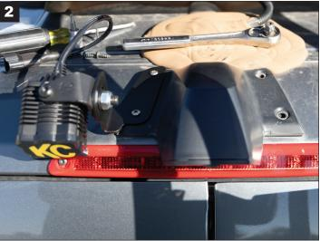
USING A T20 TORX, REMOVE THE FACTORY SCREWS FROM ONE SIDE OF THE CAMERA POD. USING THE SUPPLIED STAINLESS STEEL PHILLIPS SCREWS (#2 PHILLIP SCREW DRIVER) TO MOUNT THE FLEX ERA 1 LIGHT ASSEMBLY WITH MOUNT - MAKING SURE NOT TO OVER-TIGHTEN TO PREVENT STRRIPPING OUT THE PLASTIC THREAD BASE.
