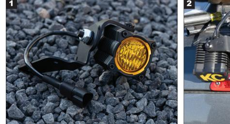
**PREP THE BACK-UP KIT INSTALLATION BY PRE-INSTALL THE FLEX ERA 1 TO THE CORRESPONDING DRIVER AND PASSENGER SIDE LIGHT MOUNTS (AS SHOWN).** NOTE: DUE TO THE ORIENTATION OF THE LIGHT, IF USING THE SPREAD BEAM, ROTATING THE LENS 90 DEGREES MAY BE REQUIRED FOR MORE DESIRABLE BEAM COVERAGE.
