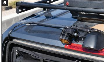
USING THE SUPPLIED ADHESIVE ZIP-TIE ANCHORS, RUN THE WIRE EXTENSION ALONG THE BACK-END OF THE REAR DRIVER-SIDE, DOWN THE DOOR SEAL.
