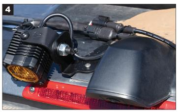
CONNECT BOTH LIGHTS TO THE SUPPLIED EXTENSION HARNESS AND SECURE THE LIGHT LEADS TO THE ZIP-TIE POINTS ON THE MOUNTING BRACKETS.
