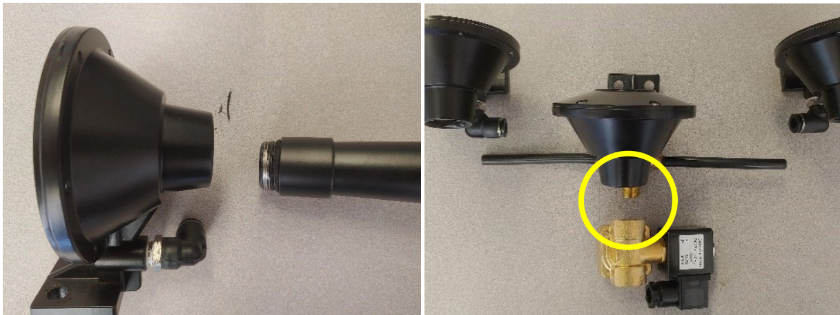
Figure 5- Trumpet Removal & Solenoid Installation
