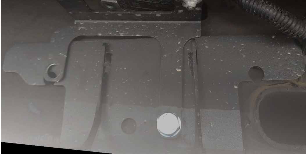
Figure 35- Compressor Bracket Installation 1, Diesel
