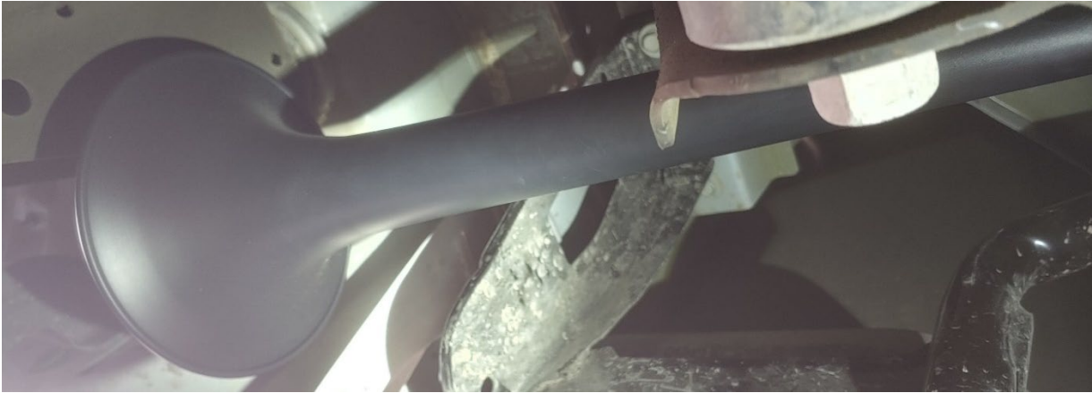
Figure 22- Trumpet Alignment to Prevent Vehicle Contact
