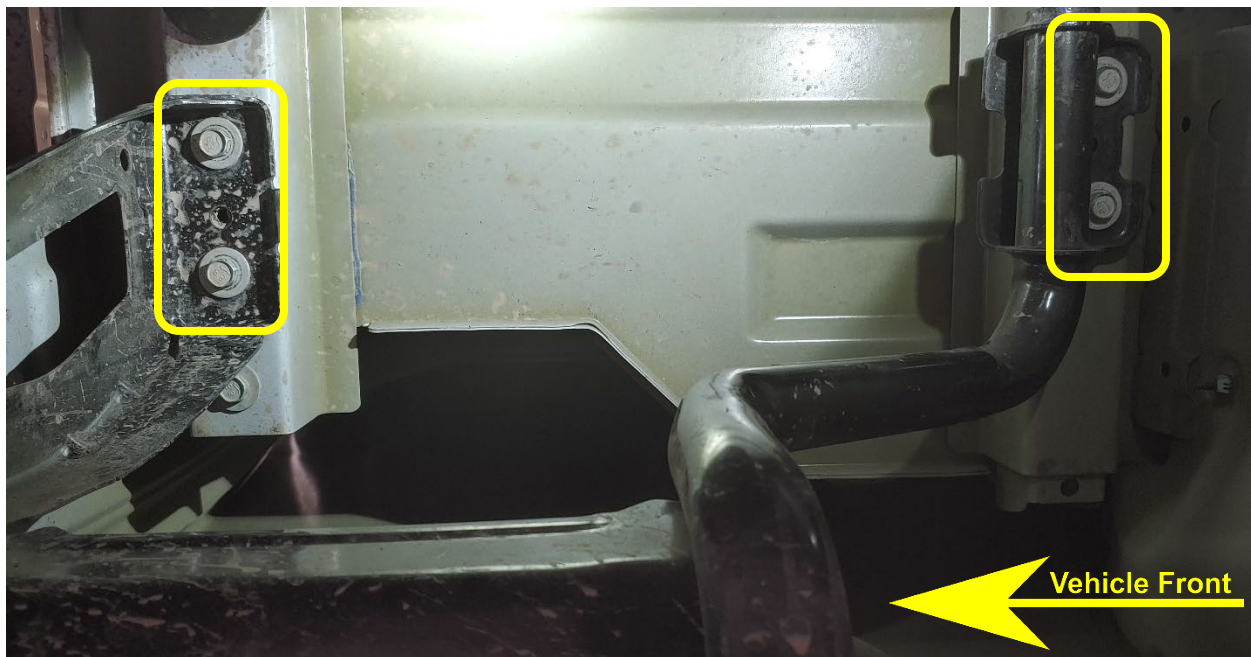
Figure 20- Passenger Side Horn Bracket, Mounting Points
