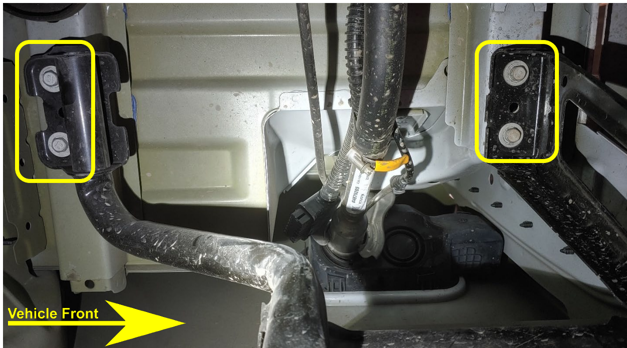
Figure 13- Driver Side Horn Bracket, Mounting Points
