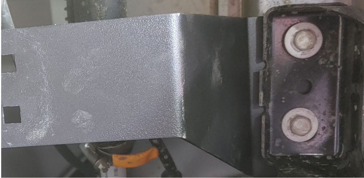
Figure 14- Driver Side Bracket Install, Frontmost Location
