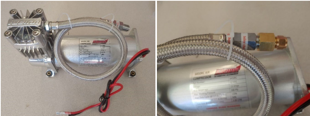
Figure 11- Compressor Fitting Installation
