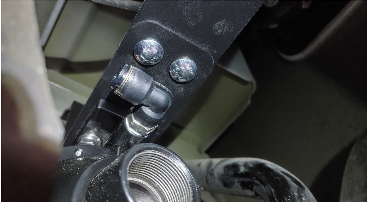
Figure 16- Driver Side Bracket Install, Brackets Temporarily Secured
