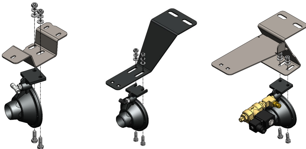
Figure 9- Air Horn Drivers, Bracket Match-Up (Center Horn Bracket, Driver Side Horn Bracket, Passenger Side Horn Bracket)
