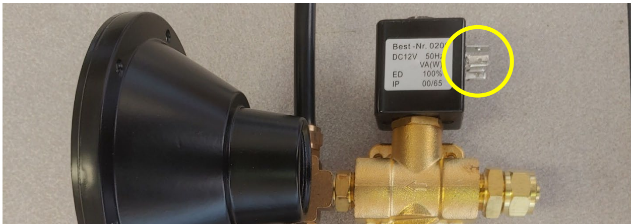
Figure 7- Solenoid Electrical Connector Removal
