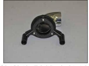
8. Install the tube with the bolts and gasket onto the tube adapter and then install the remaining gasket onto the adapter.
