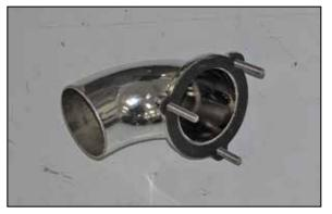
6. Install the three provided tube mounting bolts into the K&N<sup> $\otimes$ </sup> intake tube and then install one of the two provided gaskets onto the bolts.
