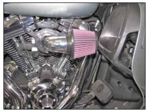
11. Install the K&N<sup>®</sup> air filter and secure with the provided hose clamp.
