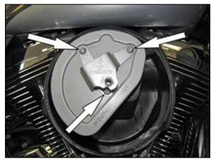
4. Remove the three bolts which secure the factory air filter to the base plate and then remove the air filter from the vehicle.
