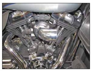
10. Install the two remaining O-Rings and K&N<sup>®</sup> breather bolts into the tube adapter. Tighten all of the hardware at this time.
