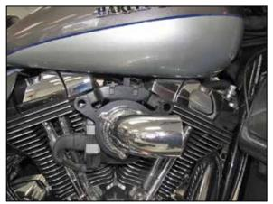
9. Apply one drop of the provided thread locker onto the tube mounting bolts. Install the complete tube and adapter assembly onto the throttle body and secure with the tube mounting bolts. **NOTE: Do not completely tighten the tube bolts at this time.**
