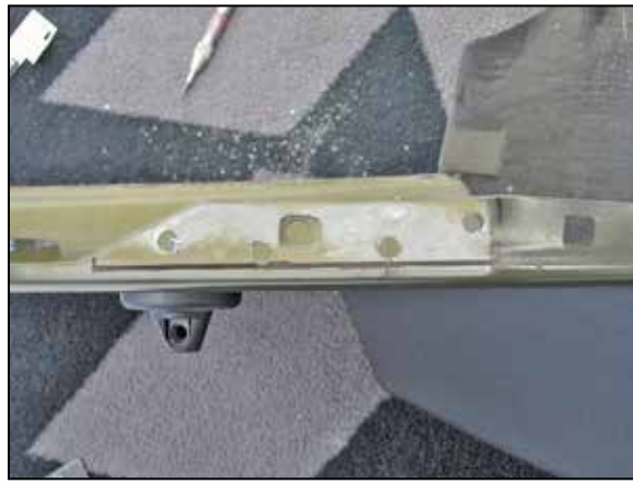
51. Using the provided template, mark the fender where the excess material needs to be removed from the fender.
