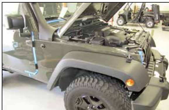
54. With an assistant, temporarily reinstall the fender onto the vehicle but do not secure it at this time. Adjust the snorkel for best fit and then secure the snorkel bracket to the inner cowl and the outer cowl to the snorkel with the factory hardware.
