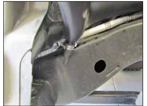
58. Install the duck bill fitting onto the port at the bottom of the corner tube and secure with the provided hose clamp.
