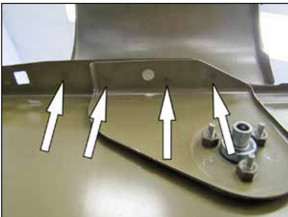
49. Use a center punch to mark the four spot welds which hold the cowl corner cap to the fender. Then drill out the spot welds to remove the cowl cap from the fender.
