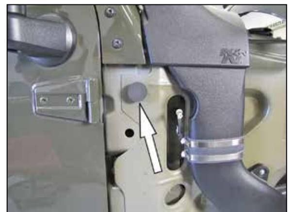
59. Peel the backing of the provided damper pad and then install it as shown on the inner body.
