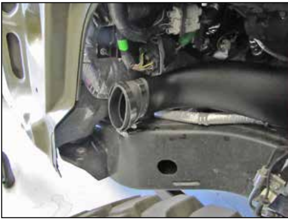
47. Install the provided coupler hose (08711) onto the lower tube and secure with the provided hose clamp.
