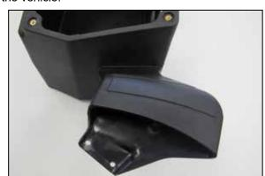
8. Install the K&N Fresh air intake duct to the K&N air filter housing and secure with the provided hardware.
