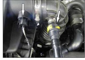
2. Disconnect the inlet air temperature sensor electrical connection and disconnect the crank case vent line from the factory intake tube.
