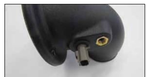
9. Remove the inlet air temperature sensor from the factory housing. Remove the O-Ring from the sensor and then install the sensor into the K&N intake tube using the provided grommet.
