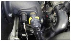
14. Reconnect the inlet air temperature sensor electrical connection and connect the crank case vent line to the fitting installed into the K&N intake tube.
