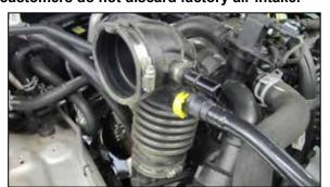
7. Loosen the hose clamp that secures the intake hose to the plenum and then remove the hose from the vehicle.
