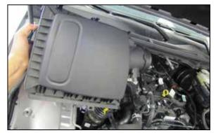
6. Remove the air filter housing from the vehicle. NOTE: K&N Engineering, Inc., recommends that customers do not discard factory air intake.
