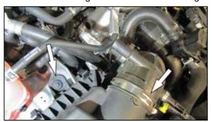
5. Remove the rear air filter housing mounting bolt and loosen the hose clamp that secures the intake hose to the housing.
