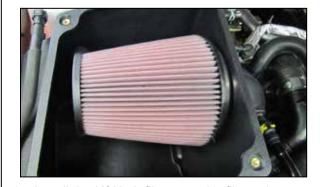
15. Install the K&N air filter onto the filter adapter and secure with the provided hose clamp.
