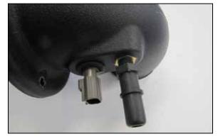
10. Install the provided crank case quick connect fitting into the K&N intake tube as shown.
