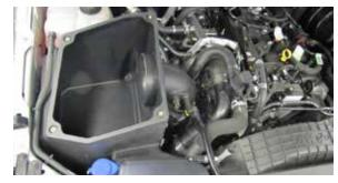
13. Install the provided Coupler hose (08711) onto the K&N intake tube and then install the complete assembly into the vehicle. Secure the housing and fresh air duct with the factory hardware and the coupler with the hose clamps provided.
