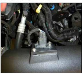
19. Reconnect the mass air sensor electrical connection.
