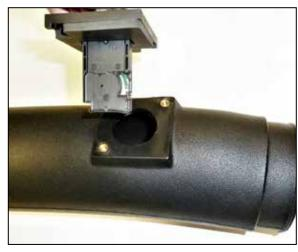
13. Install the mass air assembly into the K&N intake tube and secure with the provided hardware. NOTE: Be sure to install the sensor in the correct direction for proper operation.
