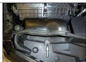
5. Remove the push pin securing the fresh air intake duct and then remove the duct from the vehicle.
