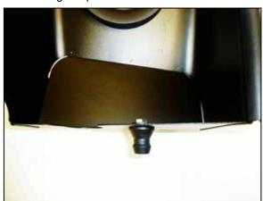
10. Install the mounting post onto the heat shield and secure with the provided hardware.
