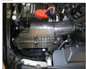
6. Pull up the air filter housing and remove it from the vehicle.
