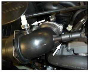
2. Disconnect the two CCV hoses from the factory intake tube. Note: Some vehicles may only have the fitting on the side of the intake tube. The manufacturer has used tow different size fitting for the top vent line.
