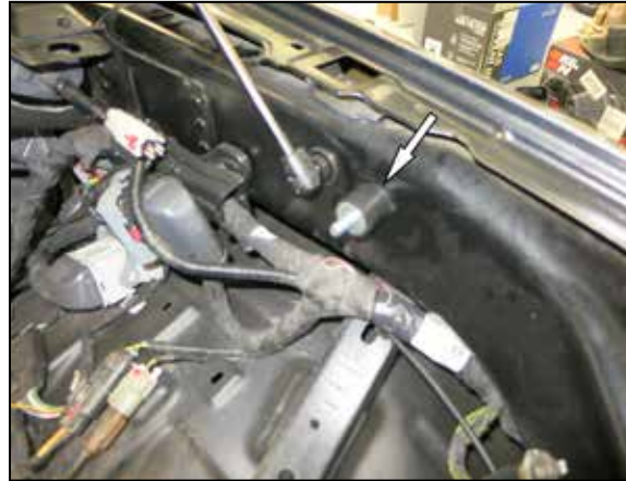
11. Install the provided rubber mounted stud into the inner fender at the air filter housing mounting location.
