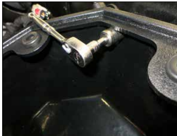
13. Secure the housing to the rubber mounted stud from step #11 with the provided hardware.
