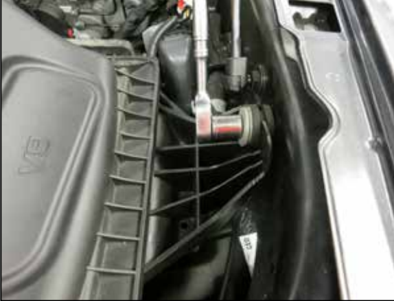
6. Remove the bolt that secures the factory air filter housing to the inner fender.
