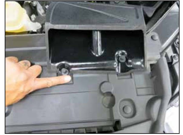
14. Secure the fresh air intake duct with the provided push pins.
