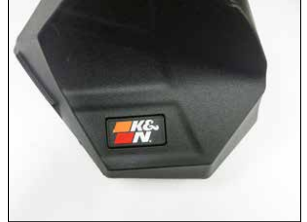
15. Snap the K&N badge into the upper air filter housing.
