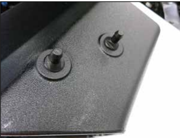
9. Install the provided mounting studs onto the K&N lower air filter housing using the provided hardware.
