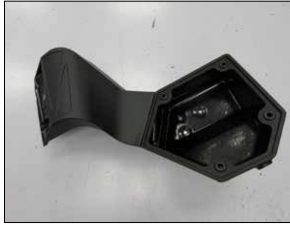
10. Install the K&N fresh air duct onto the K&N lower air filter housing using the provided hardware.
