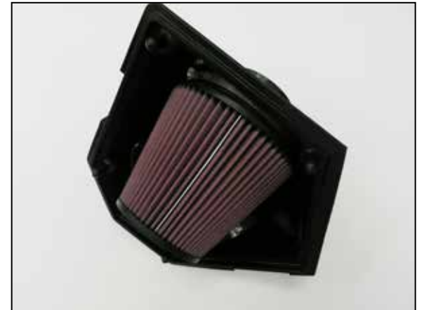
17. Install the K&N air filter onto the adapter and secure with the provided hose clamp.
