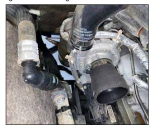
12. Install the provided step coupler onto the passenger side turbo inlet and secure with the provided hose clamp.
