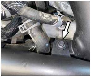
6. Remove the bolt shown that secures the drivers side intake tube to the cold-side charge tube and then remove the drivers side intake tube from the vehicle.
