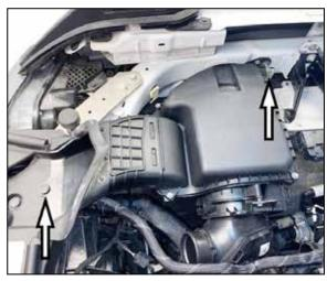
7. Remove the push-pin that secures the fresh air inlet. Remove the air filter housing mounting bolt.
