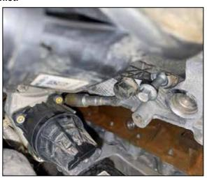
11. Reinstall the intake tube mounting bolt into the original location and tighten.
