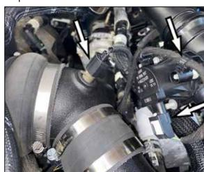
25. Reconnect the IAT sensor and BOV electrical connections and secure the BOV harness to the
