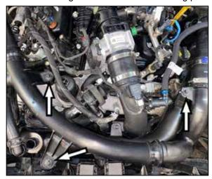
4. Remove the three mounting bolts securing the factory charge tube to the engine. Loosen the hose clamp that secures the right side of the charge tube and then release the two spring clamps and remove the factory charge tube from the vehicle.
