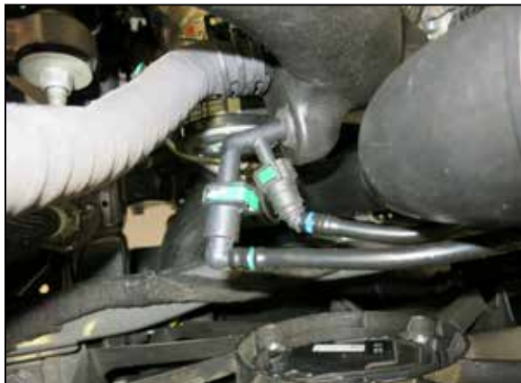
25. Reconnect the Ejector hoses onto the ejector installed into the K&N intake tube.
