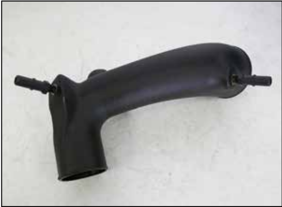
17. Install the two provided quick connect fittings into the K&N intake tube as shown.
