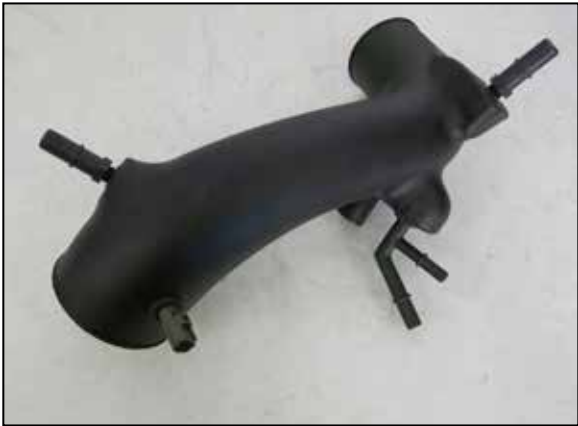
20. Remove the O-ring from the IAT sensor and then install it into the remaining grommet installed into the K&N intake tube.
