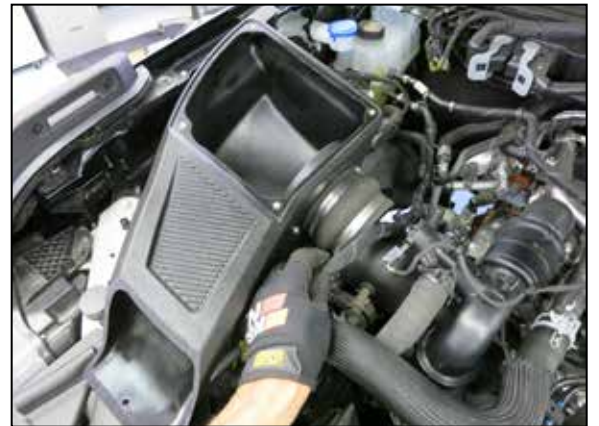
29. Install the K&N air filter housing assembly into the vehicle.
