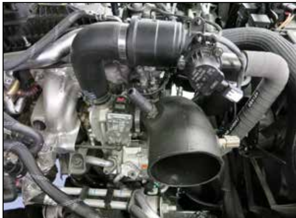
23. Install the K&N intake tube assembly onto the turbo inlet but do not secure the hose clamp.
