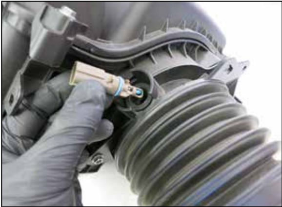
19. Rotate the IAT sensor counterclockwise and up to remove it from the factory air filter housing.
