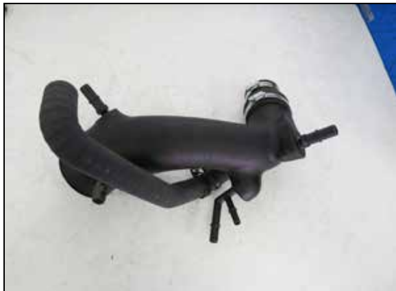
22. Install the provided BOV with factory clamps onto the K&N intake tube.
