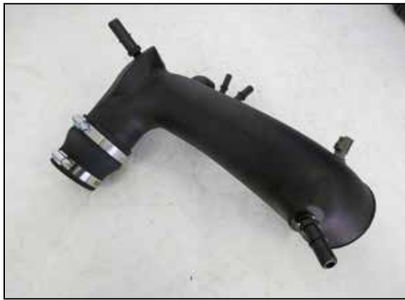
21. Install the provided step coupler onto the K&N intake tube and secure with the provided hose clamp.
