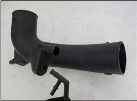
18. Install the provided Ejector fitting into the grommet in the K&N intake tube as shown.
