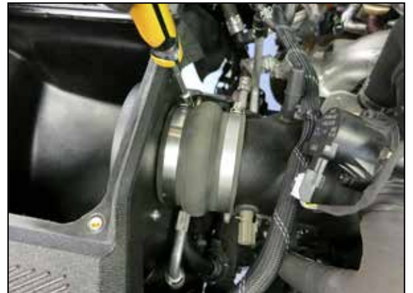
30. Connect the intake tube to the coupler and secure with the hose clamp.
