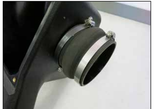
28. Install the provided filter adapter into the K&N air filter housing and secure with the provided hardware. Install the provided hump coupler onto the filter adapter and secure with the hose clamp.
