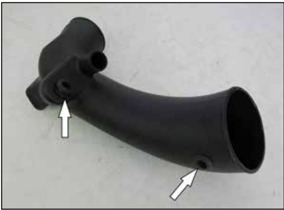
16. Install the two provided grommets into the K&N intake tube where shown.
