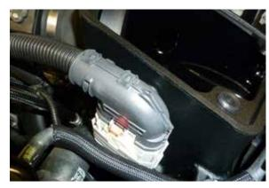
19. Install the wiring harness bulk connector onto the bracket installed onto the K&N air filter housing.
