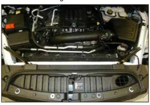
34. Reinstall the upper radiator valence and secure with the ten factory push pins.
