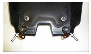
27. Using the factory bolts and the nuts provided, secure the two provided "Z" brackets to the engine cover as shown.
