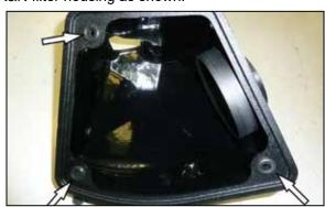
16. Install the three provided grommets into the K&N air filter housing as shown.
