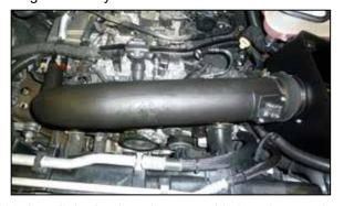
26. Install the intake tube assembly into the coupler at the air filter housing and then into the coupler at the turbo inlet, adjust the tube for best fit and then secure with the provided hose clamps.
