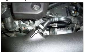
29. Connect the CCV tube to the guick connect fitting installed into the K&N intake tube.
