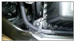
12. Remove the nut that secures the air filter housing to the mounting bracket. This nut will be reused in a later step.
