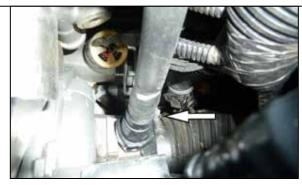
5. Loosen the hose clamp that secures intake tube to the turbo inlet.
