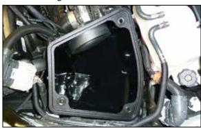
17. Install the K&N air filter housing into the vehicle and secure with the factory nut from step #12.
