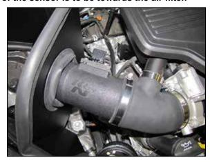
12. Install the K&N® intake tube assembly into the heat shield and coupler.
