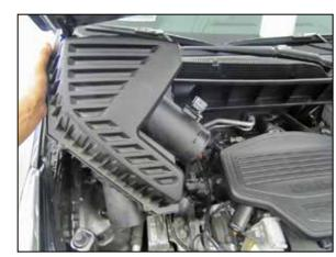
5. Pull up the factory air filter housing to dislodge it from the mounting grommets and then remove the housing from the vehicle. NOTE: K&N Engineering, Inc., recommends that customers do not discard factory air intake.
