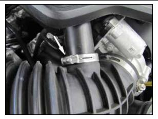
3. Pry loose the band clamp that secures the intake plenum tube to the intake hose and remove the
