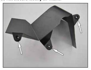
6. Remove the three mounting grommets from the factory air filter housing and install them into the K&N® heat shield as shown.
