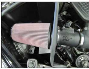
13. Install the air filter onto the intake tube, adjust the intake tube and filter for best fit and then secure the hose clamp.
