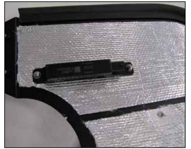
24. Install the "F" antenna to the engine side of the driver's side heat shield assembly using the provided hardware with the button head of the bolt on the filter side of the heat shield.
