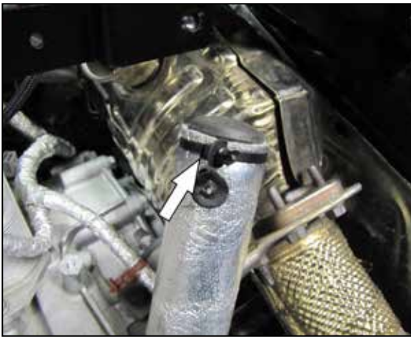
16. If the Transmission reservoir mount broke during disassembly, Install the mounting tree tie wrap onto the reservoir as shown.
