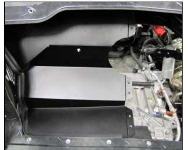
25. Install the drivers side heat shield assembly and align with the mounting bracket. Secure the heat shield with the provided hardware. Reconnect the "F" antenna electrical connection.
