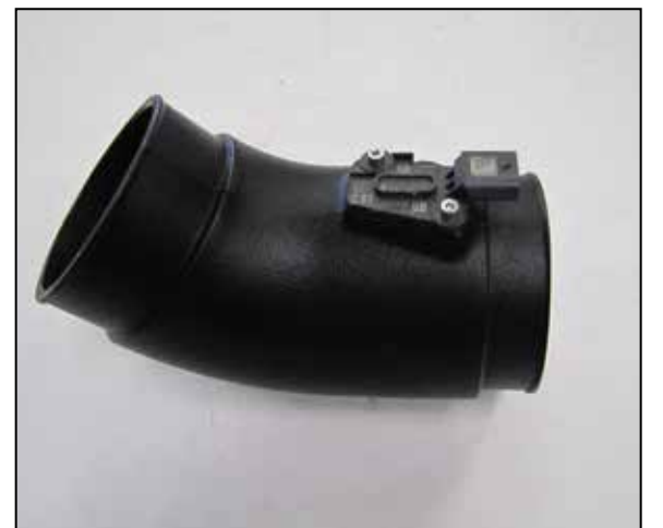
26. Remove the mass air sensor from the factory air filter housing and install it into the K&N intake tube using the provided hardware.
