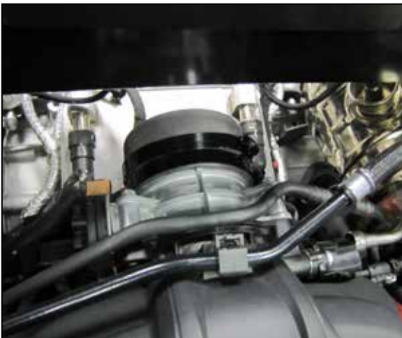
18. Install the coupler onto the throttle body and secure with the provided hose clamp.
