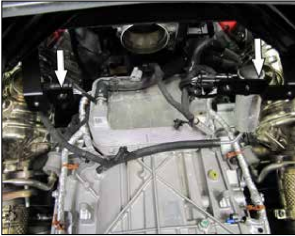
17. Attach the transmission vent reservoir and O2 wiring harness to the heat shield mounting brackets.
