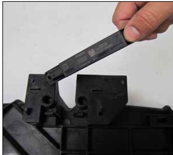
22. Cut the sonic welds that secure the "F" antenna to the air filter housing and then remove the antenna from the housing.
