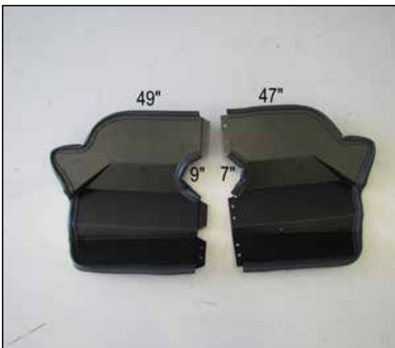
20. Install the provided edge trim onto the two heat shield halves as shown.
