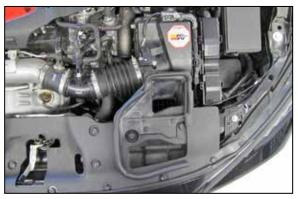
2. Disconnect the mass air sensor electrical connection and unhook the harness from the air filter housing.
