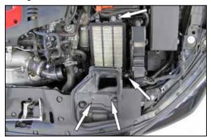
4. Remove the four bolts that secure the lower air filter housing and fresh air scoop and then remove the complete assembly from the vehicle.
