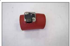
11. Remove the mass air sensor from the factory housing and install it into the K&N® intake tube as shown.
