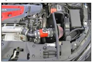
14. Install the intake tube assembly onto the turbo inlet and filter adapter, adjust the tube for best fit and secure with the provided hose clamp. NOTE: Be sure the tube is in the correct
