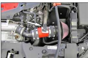
15. Remove the plastic harness holder from the mass air sensor harness. Install the provided split harness cover and secure with electrical tape. Route the harness through the notch in the front of the heat shield and then reconnect the mass air sensor electrical connection.
