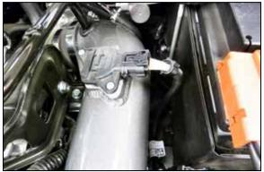
13. Reconnect the mass air sensor electrical connection.
