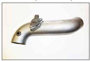
11. Remove the mass air sensor from the factory housing and then install it into the K&N intake tube using the factory screws. Install the provided PCV grommet into the K&N intake tube as shown.
