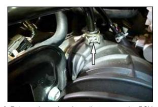
2. Release the spring clamp that secures the PCV pipe and then disconnect the pipe from the factory intake tube.
