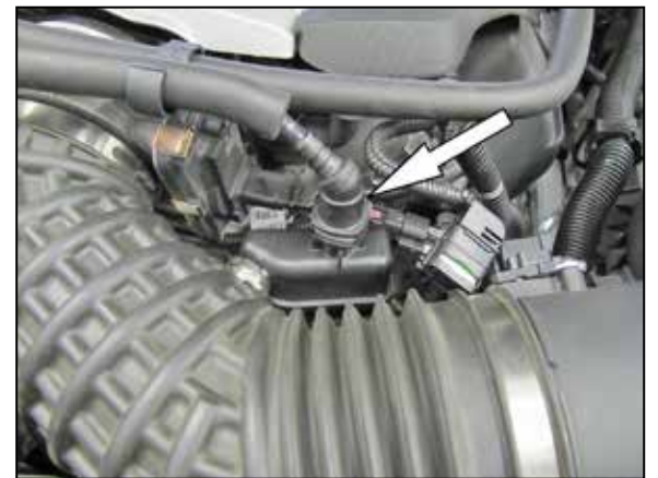
3. Disconnect the crank case vent quick connect fitting from the intake tube.
