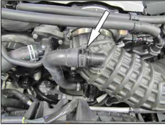
4. Release the spring clamp securing the sound tube to the fitting in the intake tube and then disconnect the sound tube.
