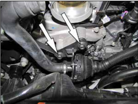
6. Remove the two bolts securing the sound drum to the front of the engine.
