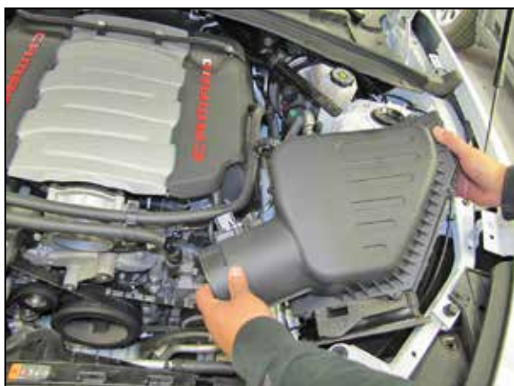
12. Lift up the air filter housing to dislodge it from the mounting grommets and then remove it from the vehicle.
