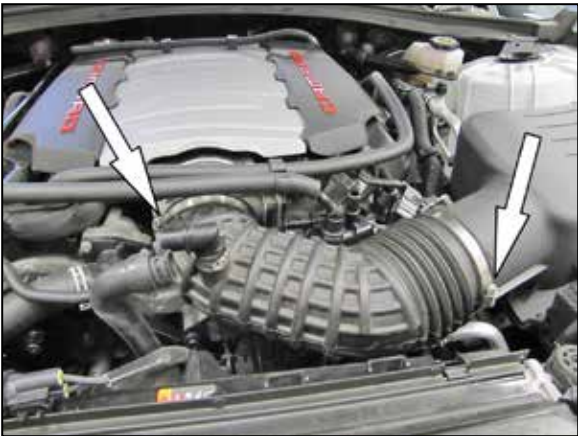
5. Loosen the hose clamps securing the intake tube to the throttle body and air filter housing and then remove the intake tube.
