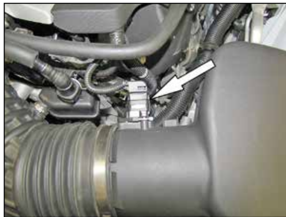
2. Disconnect the mass air sensor electrical connection.
