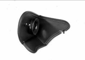
15. Install remaining mounting post onto the long leg of the provided bracket (064340) and then install the assembly onto the heat shield using the provided hardware.
