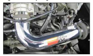
26. Install the provided crank case vent hose onto the factory vent hose and K&N<sup>®</sup> fitting.
