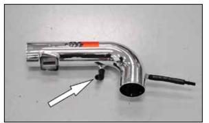
11. Remove the factory crank case vent coupler from the crank case vent tube. **NOTE: Us twisting/pulling motions to slip the coupler off the tube, it is not necessary to cut the factory clamp.**
