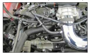
25. Connect the K&N<sup>®</sup> EVAP quick disconnect fitting into the factory fitting.
