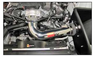
24. Install the K&N<sup>®</sup> intake tube assembly into the coupler at the filter adapter and then into the coupler on the throttle body, adjust the tube for best fit and then secure with the provided hose clamps.
