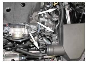
6. Release the three flexible clamps that secure the sound tube and disconnect the sound drum from the rear sound tube then remove the sound tube assembly.
