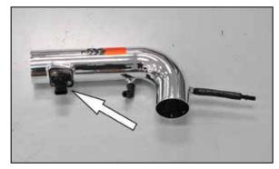
23. Install the mass air assembly into the  $K\&N^{\circledast}$  intake tube as shown.
