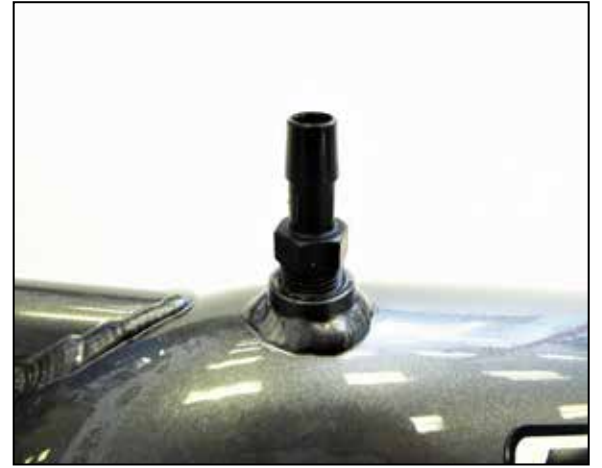
14. Install the provided vent fitting into the K&N intake tube as shown.
