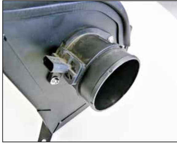
9. Using the provided hardware attach the mass air sensor to the heat shield as shown.
