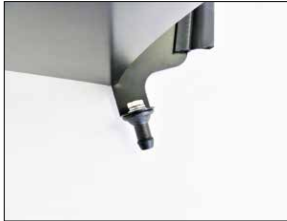
10. Install the mounting stud to the heat shield as shown.
