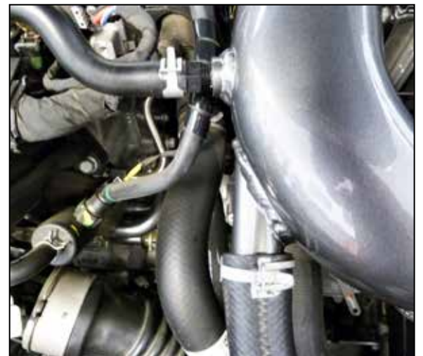
16. Connect the BOV hose and the vent line and secure with the provided spring clamp.
