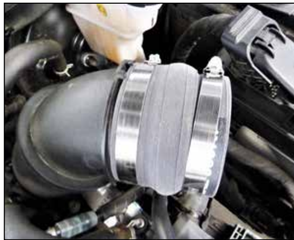
12. Install the provided hump coupler onto the turbo inlet and secure with the provided hose clamp.
