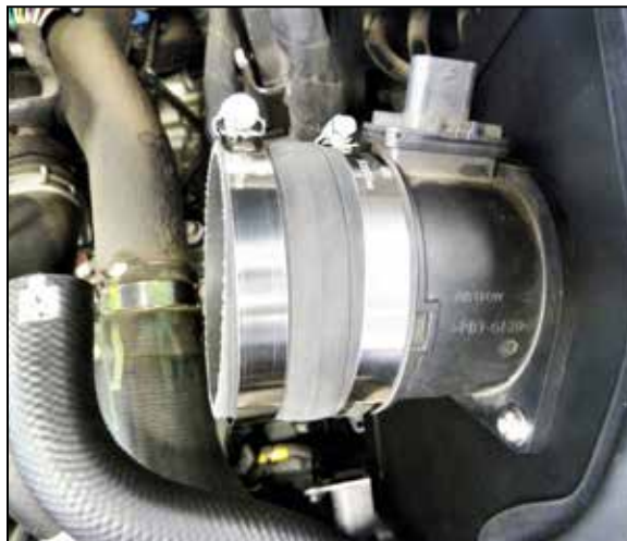
13. Install the provided straight coupler onto the mass air sensor and secure with the provided hose clamp.
