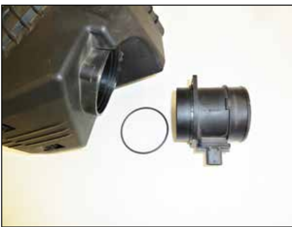
7. Remove the mass air filter from the factory air filter housing and then remove the O-ring seal from the sensor.
