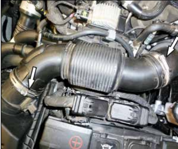
5. Loosen the two hose clamps that secure the factory intake tube and then remove the tube from the vehicle.
