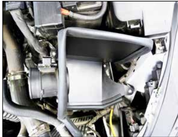
11. Install the heat shield assembly into the vehicle so the mounting stud inserts into the mounting grommet, then secure with the provided hardware.
