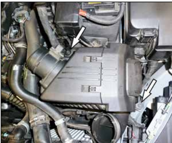
6. Remove the two bolts that secure the air filter housing and then remove the filter housing from the vehicle.
