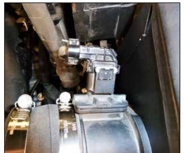
17. Reconnect the mass air sensor electrical connection.
