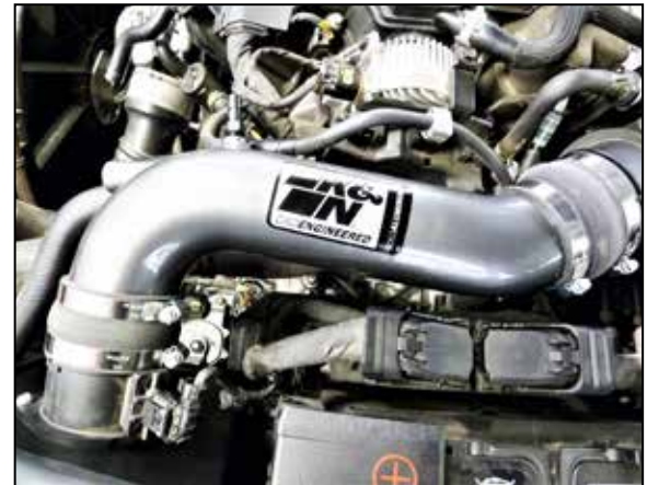
15. Install the intake tube into the hump coupler and then into the straight coupler, adjust for best fit and then secure with the provided hose clamps.
