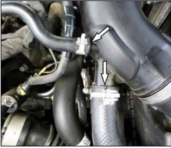
4. Release the spring clamps that secure the BOV hose and vent line, then disconnect the lines from the factory intake tube.
