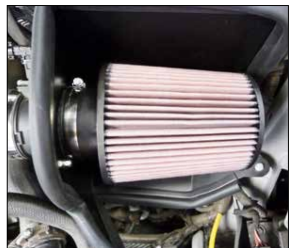
18. Install the air filter onto the mass air sensor and secure with the provided hose clamp.
