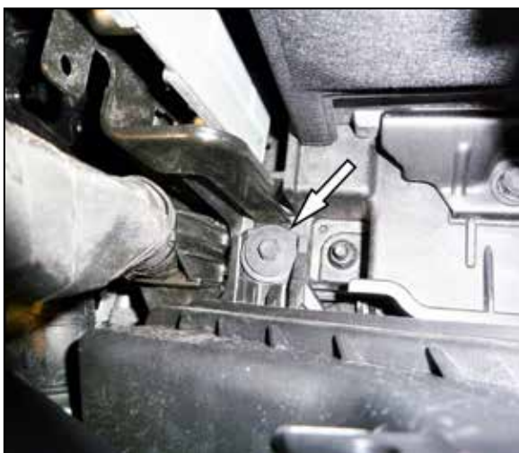
8. Remove the rear air filter housing mounting bolt and then remove the air filter housing from the vehicle.
