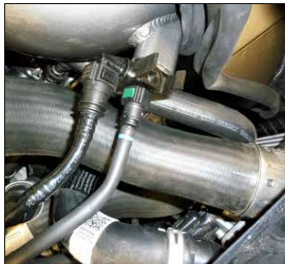
18. Reconnect the Ejector fitting vent line connections.
