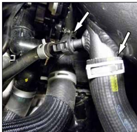
17. Connect the BOV hose and the vent line with the installed straight fitting onto the K&N intake tube as shown.
