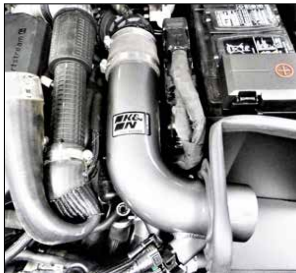
16. Install the K&N intake tube through the heat shield and into the coupler, align for best fit and then secure with the provided hose clamp.
