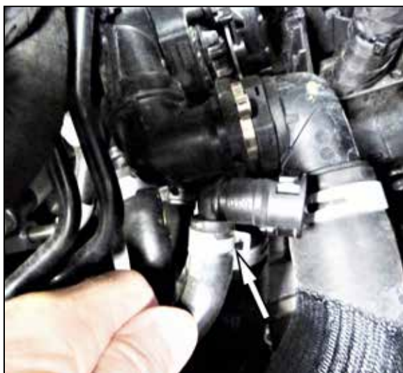
13. Release the spring clamp that secure the 90degree quick connect fitting from step #5 and then remove the fitting and replace it with the straight quick disconnect fitting provided.
