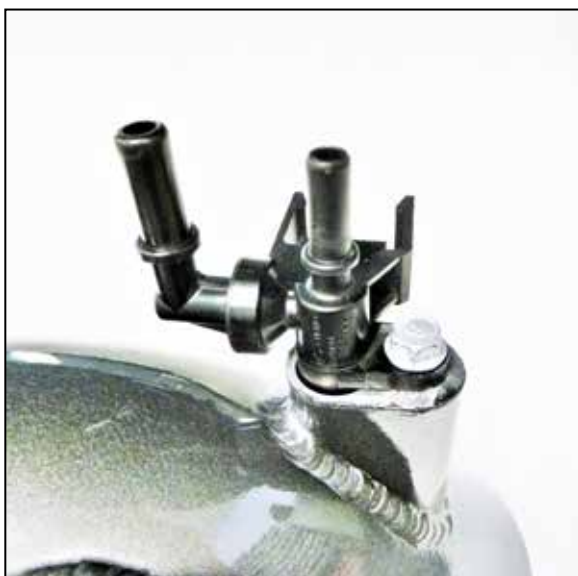
10. Install the ejector fitting onto the K&N intake tube using the factory bolt.
