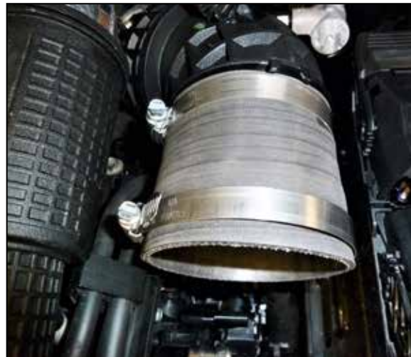
15. Install the provided coupler onto the turbo inlet pipe and secure with the provided hose clamp.
