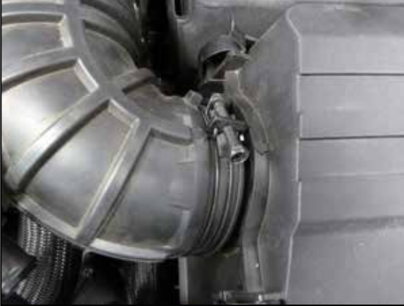
5. Loosen the hose clamp that secures the factory intake tube to the air filter housing and then remove the intake tube from the vehicle.
