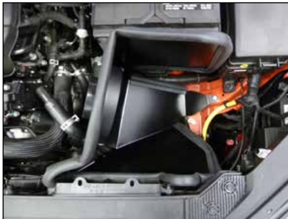
11. Install the heat shield assembly into the vehicle and secure with the provided hardware.
