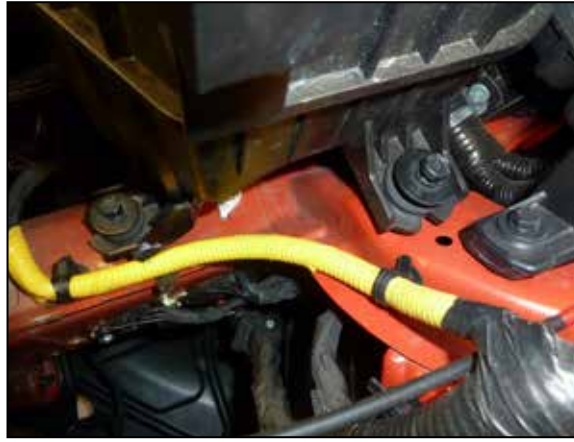
8. Remove the two remaining air filter housing mounting bolts and then remove the air filter housing from the vehicle.
