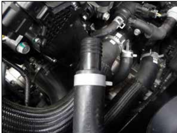
12. Install the BOV hose union into the factory BOV hose and secure with the factory spring clamp.
