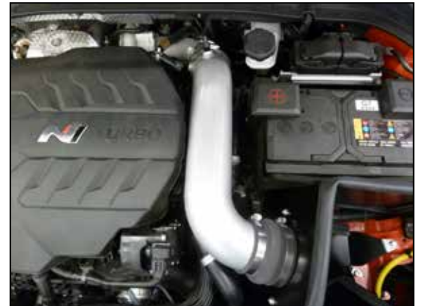
17. Install the K&N intake tube into the coupler at the turbo inlet and then into the hump coupler, adjust the tube for best fit and then secure with the provided hose clamps.
