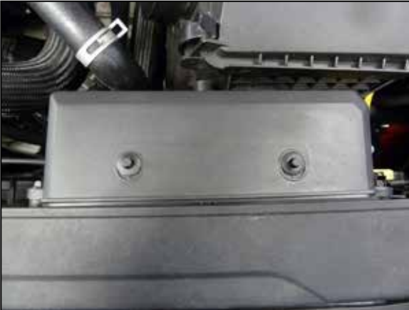
6. Release the centers of the retaining pins that secure the fresh air duct and then remove the pins.
