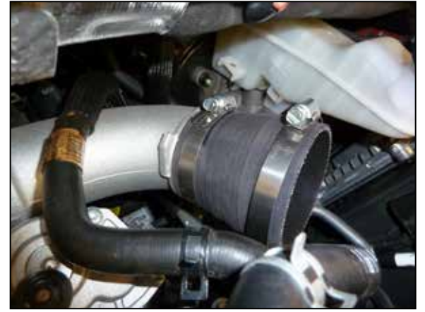
13. Install the step coupler onto the turbo inlet and secure with the provided hose clamp.
