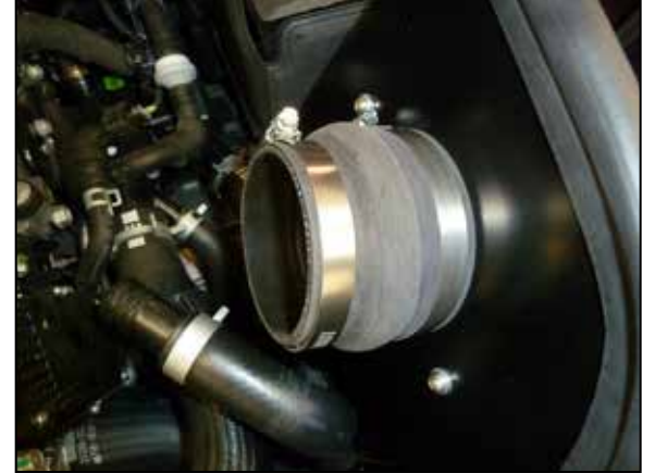
14. Install the hump hose onto the filter adapter and secure with the provided hose clamp.
