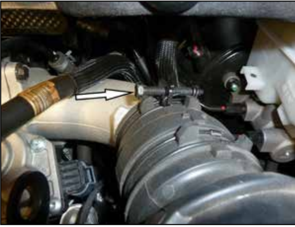
4. Loosen the hose clamp that secures the factory intake tube to the turbo inlet.
