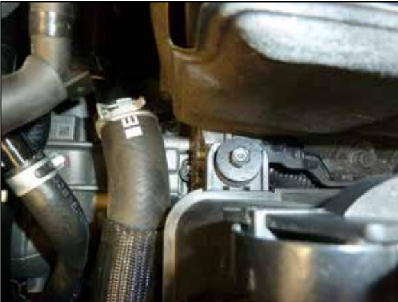
7. Remove the rear air filter housing mounting bolt.
