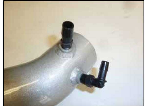
15. Install the provided CCV and EVAP fittings into the intake tube as shown. Apply pipe thread sealant to the threads before installation.
