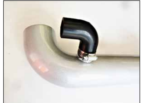
16. Cut 9" off the straight section of the provided BOV hose and then install the 90-degree section onto the intake tube and secure with the provided hose clamp.
