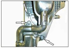
6. Remove the two push-pins that secure the fresh air duct to the air filter housing, release the locking tab and then rotate the duct counter clockwise to remove it from the air filter housing.
