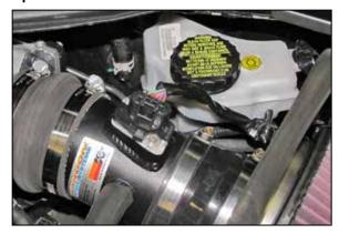
24. Reconnect the mass air sensor electrical connection.
