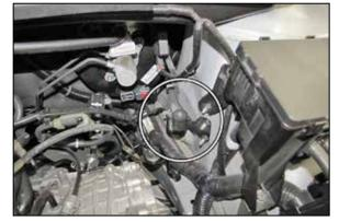
9. THIS STEP IS FOR THE NISSAN PATHFINDER AND INFINTI JX35 VEHICLES ONLY. Install the remaining 1" tall, male/female rubber mounted stud onto the air box mounting bracket as
