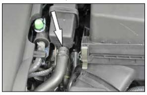
4. Release the spring clamp securing the crank case vent hose to the intake plenum and then disconnect the crank case vent hose.
