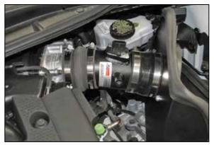
19. Install the K&N<sup>®</sup> intake tube into the hump hose, Pull the heat shield forward and install the intake tube into the hose at the filter adapter. Adjust the tube for best fit and then secure the tube with the provided hose clamps.
