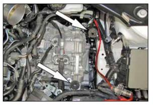
7. Remove the two air box mounting grommets shown from the mounting brackets.
