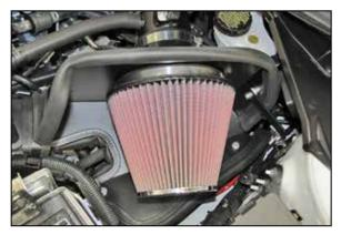
23. Install the K&N<sup>®</sup> air filter onto the filter adapter and secure with the provided hose clamp. NOTE: Drycharger<sup>®</sup> air filter wrap; part # RF-1048DK is available to purchase separately. To learn more about Drycharger<sup>®</sup> filter wraps or look up color availability please visit http://www.knfilters.com<sup>®</sup>.
