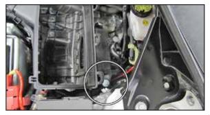
6. Remove the bolt which secures the lower air box to the mounting bracket. Remove the lower air box from the vehicle.
