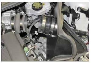
16. Install the provided coupling hose (08051) onto the filter adapter and secure with the provided hose clamp.
