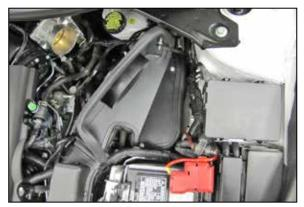
14. Install the heat shield assembly onto the rubber mounted studs. Secure the heat shield with the provided hardware. Clip the transmission vent into the hole in the heat shield.
