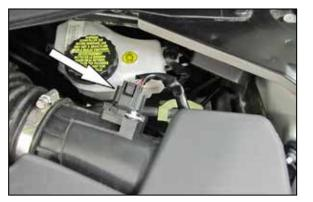
2. Disconnect the mass air sensor electrical connection and unhook the wiring harness from the air box.
