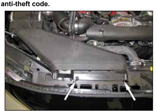
2. Remove the two plastic retaining clips that secure the fresh air duct and then remove the fresh air duct from the vehicle.
