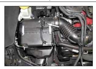
3. Disconnect the mass air sensor electrical connection and unclip the wiring harness from the air filter housing.
