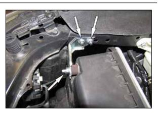
5. Remove the three nuts that secure the air filter housing to the inner fender and then remove the bracket from the vehicle.
