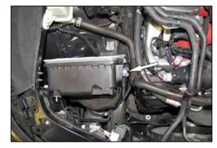
6. Remove the bolt that secures the dirty side air filter housing to the frame rail and then remove the air filter housing from the vehicle.
