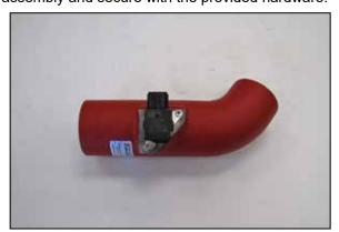
11. Remove the mass air sensor from the factory air filter housing and install it into the K&N® intake tube using the provided hardware.
