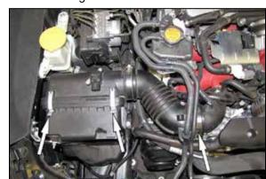
4. Loosen the hose clamp that secures the intake hose to the turbo inlet. Release the air filter housing clam shell clips and then remove the air filter clean side housing, intake hose and factory air filter from the vehicle.
