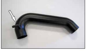
18. Install the provided 90° vent fitting into the K&N^ ${\ensuremath{\mathbb S}}$  intake tube as shown.
