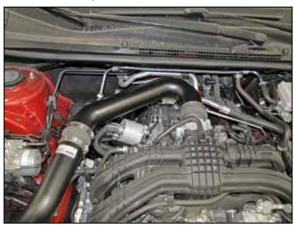
19. Install the K&N<sup>®</sup> intake tube into the hump couplers, adjust both tubes for best fit and then secure the hose clamps and the tube mount to the heat shield.
