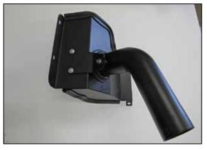
12. Install the K&N<sup>®</sup> intake tube assembly into the heat shield and secure with the provided hardware as shown but do not completely tighten at this time.
