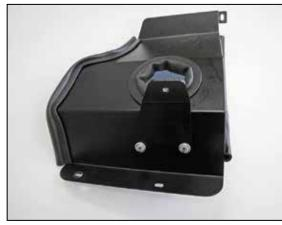
9. Install the tube mounting bracket (064336) onto the heat shield and secure with the provided hardware.
