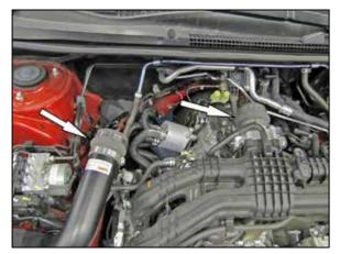
17. Install the provided hump coupler hoses onto the throttle body and the K&N<sup>®</sup> intake tube as shown and secure with the provided hose clamps.
