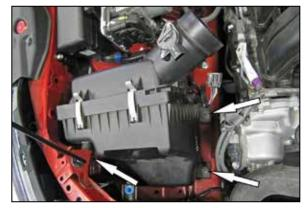
6. Remove the one nut and two bolts that secure the air filter housing and then remove the housing from the vehicle.
