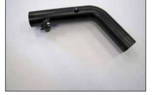
11. Install the mass air sensor into the  $K\&N^{\otimes}$  intake tube and secure with the hardware provided.
