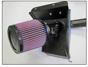
13. Install the K&N $^{\circ}$  air filter onto the intake tube and secure with the provided hose clamp.
