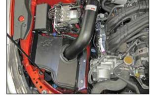
16. Plug in the mass air sensor electrical connection and then install the heat shield/tube assembly onto the rubber mounted studs and align with the electrical junction block. Secure the heat shield with the provided hardware and the factory bolt removed in step #15.
