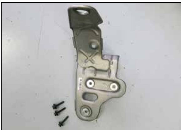
9. Remove the three bolts that secure the air filter mounting bracket and then remove the bracket from the vehicle.
