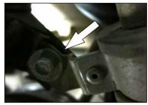
7. Remove the bolt that secures the upper part of cold side charge tube to the mounting bracket.
