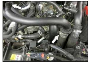
2. Loosen the hose clamps that secure the hot side upper charge tube to the turbo and hot side lower charge tube.
