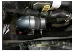
16. Install the provided hump coupler onto the lower charge tube and secure with the provided clamps.
