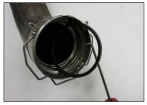
10. Remove the seal and retaining clip from the factory charge tube quick connect coupler to be used in the K&N quick connect coupler. NOTE: Pay close attention to the direction the seal is installed into the fitting.
