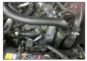
21. Reinstall the hot side upper charge tube and secure with the factory clamps.
