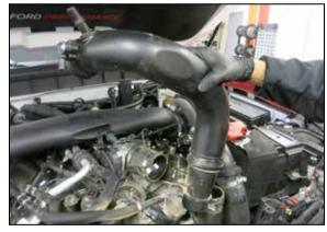
8. Remove the upper cold side charge tube from the vehicle.
