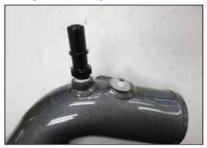
13. Install the provided CCV quick connect fitting and 1/8npt plug into the K&N charge tube.
