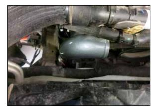
15. Install the K&N lower charge tube into position from under the vehicle and connect to the inter cooler. Push the quick connect fitting onto the inter cooler until a "click" is heard as the retaining clip locks into position. Pull back on the tube to be sure it is locked into position.
