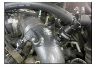
19. Reconnect the pressure sensor electrical connection and connect the CCV hose to the fitting installed into the K&N charge tube.
