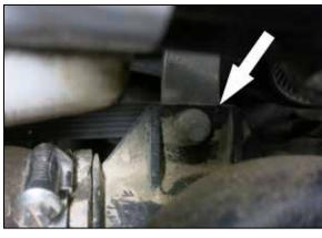
6. Remove the bolt that secures the lower part of cold side charge tube to the mounting bracket.
