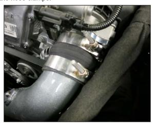
10. Install the K&N charge tube assembly and connect the intercooler connection and throttle body adapter. Push the intercooler connection until you hear the retaining clip audible "click" into its locked position. Position the hump coupler and secure with the provided hose clamps.
