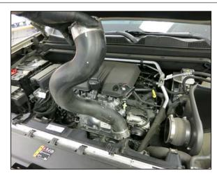
3. Pull back the locking clip that secures the charge tube coupler to the intercooler by pulling the clip back and locking into the tabs on the coupler. Then disconnect the charge tube and remove it from the vehicle.
