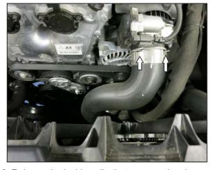
2. Release the locking clip that secures the charge tube coupler onto the throttle body by pulling the clip back and locking into the tabs on the coupler. NOTE: The intake tube is removed for photo clarity.
