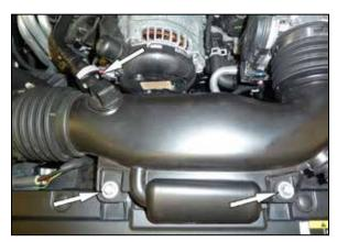
3. Remove the two bolts shown that secure the intake tube to the core support. Push the white locking for the crank case vent line down and then disconnect the crank case vent line from the intake tube.
