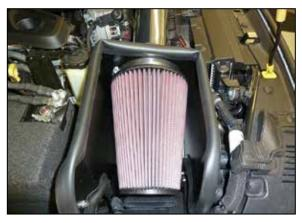
14. Install the K&N $^{\!0}$  air filter and secure with the provided hose clamp.
