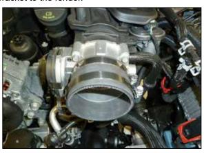
6. Install the provided coupler (08690) onto the throttle body and secure with the provided hose clamp.
