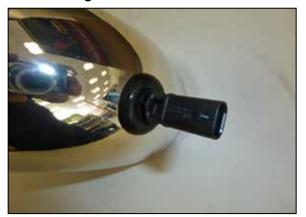
8. Install the provided grommet and factory temp sensor onto the  $K\&N^{\otimes}$  intake tube.
