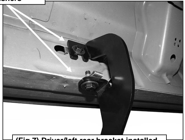
(Fig 7) Driver/left rear bracket installed
