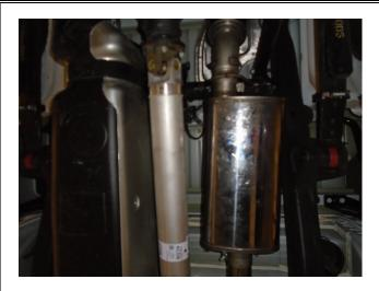
**Step 3.** Install the Muffler to the Inlet Pipe Assembly/Extension Pipe using the supplied 3.50" clamp.
