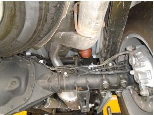
**Step 1.** To remove the OEM exhaust system, you will to need to cut the pipe behind the muffler before it goes over the axle. Disengage the welded hangers from the rubber insulators and remove the tailpipe. Next remove the fasteners from the two bolt fange behind the catlytic converter. Do not damage or discard the fasteners or rubber insulators, as they will be re-used to mount the new system. Disengage the remainder of the hangers and remove the system.
