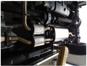
**Step 2.** Next, loosen all factory pipe clamps and disengage the welded hangers from the rubber isolators. Retain all mounting hardware as it will be needed to mount your new MAGNAFLOW system.
