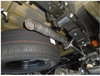
**Step 5.** Loosely install the Over Axle Pipe and Tail Pipe Assembly using the supplied clamps.
