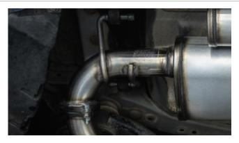
**Step 3.** Install flat gasket between Muffler and Midpipe, and insert bolts. This will position the slip fit between the Resonator and Midpipe correctly.
