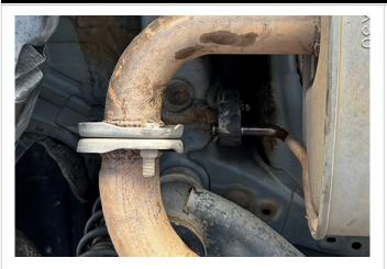
**Step 1**. Begin removal of your OEM Muffler Assembly by unbolting the flange fasteners and disconnecting the rubber insulators that suspend the Assembly (see above). The Muffler Assembly can now be removed. Do not damage or discard the rubber insulators as they will be used to Install the new system
