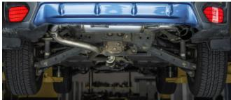
**Step 4.** Once proper positioning has been attained for the new exhaust system, tighten the clamp and fasteners using the torque specification on page one of these instructions. Inspect all clamps and flasteners after 25-50 miles of operation. Re-tighten if necessary.
