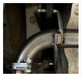
**Step 2.** Install the MagnaFlow muffler assembly into the empty space near the rear bumper. For easiest installation, begin with the rear driver's side insulator.
