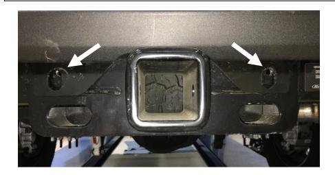
**4.** Remove the (x4) Nuts that attach the bumper to the frame brackets and carefully remove the bumper and set aside.
