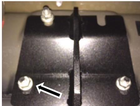
**Step 7.** After final adjustment, tighten all four brackets at the main tube.
