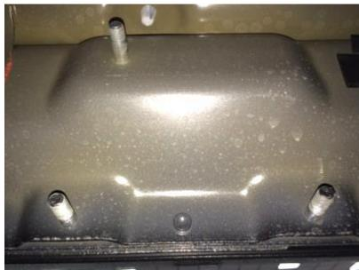
**Step 4.** Carefully raise step into position and align the three brackets with the threaded studs.
