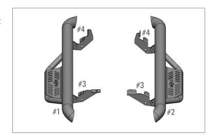
NOTE: Brackets will attach to the backside of the mounting flange with the threaded end of the (#7) carriage bolt (x2) facing towards the rear of the step.
