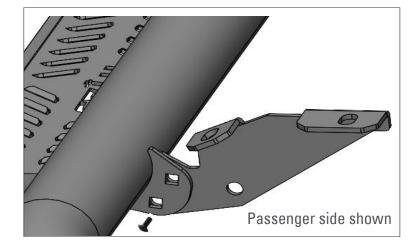
Step 2. Remove any factory running board/steps and hardware and discard.
