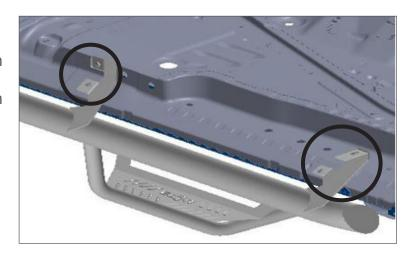
Step 7. Finish by tightening the (x2) carriage bolt/nut (#7,#6) mounting brackets at the main tube. (20-25 ft./lbs. torque). Step 8. Repeat process with passsenger side.
