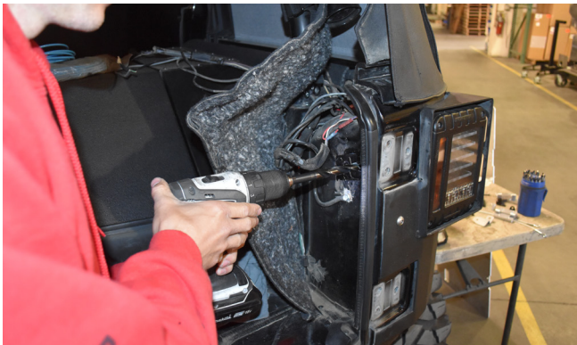
Drill the hole to 17/32".
