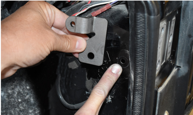
Drill the hole to 17/32".
