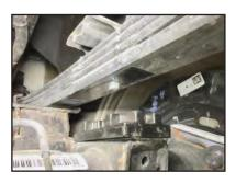
**STEP 8:** Install lift block, 1.5" height shown.
