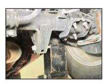
**STEP 4:** Loosen and remove OEM ubolts, nuts and plate.
