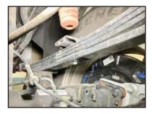
**STEP 6:** Install tapered lift block with 'FRONT' marking towards front of vehicle.
