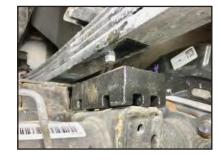
**STEP 9:** Install lift block, 2.0" height shown.
