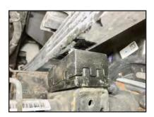
**STEP 10:** Carefully lower vehicle until spring rests upon lift block. Make sure the spring alignment stud fits inside block alignment hole.
