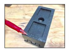
**STEP 7:** Install lift block, 1.0" height shown.
