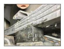
**STEP 11:** Install new Ubolts provided with the kit. Install spring bracket and install washers and nuts.
