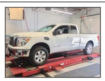
**STEP 2:** On a flat, level surface, MEASURE preinstallation ride height, FRONT & REAR, and write down measurements. Front (L)
