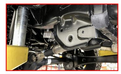
Install the replacement radius arm to axle using factory hardware for the upper connection and using the supplied cam bolts for the lower connection.
