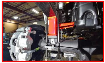
Install rear Falcon shock using factory hardware.
