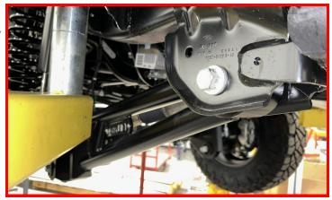
At this time, align the cam bolts as described below and torque to 200 ft-lbs. It is recommended to check alignment and make adjustments to cams before applying final torque.
