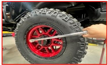
Re-check all hardware (both the front and the rear) for proper installation and torque.
