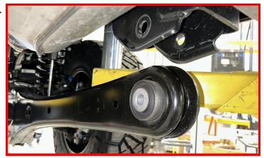
Remove the (2) radius arm axle mounting bolts.
