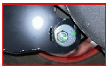
Tighten the upper axle mount radius arm bolt.
