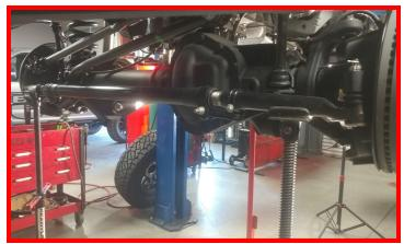
Remove the factory radius arm pivot hardware.
