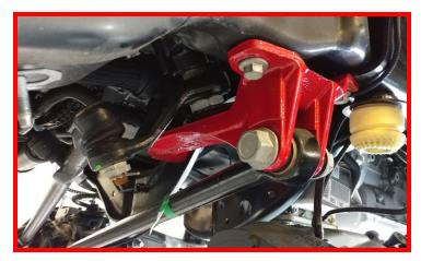
Install the ReadyLIFT sway bar drops to the frame using factory hardware.
