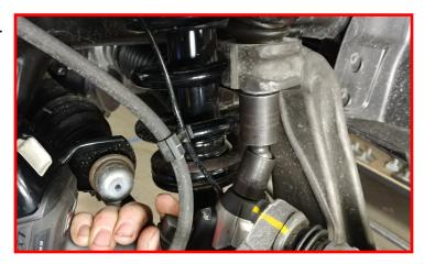
Strike the upper ball joint boss on knuckle with a dead blow hammer to dislodge the taper.
