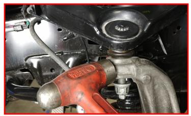
Remove the factory upper control arm from the frame.
