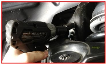
Remove the ABS wire harness from the upper control arm and frame rails. Cut the Christmas tree clip off the harness.
