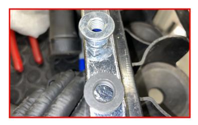
Attach the upper control arm ball joint to the knuckle using the provided hardware.
