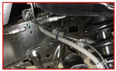
Connect the vehicles power source at the negative ground terminal.
