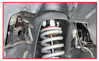
Install the appropriate side control arm to the frame rail using the factory hardware.
