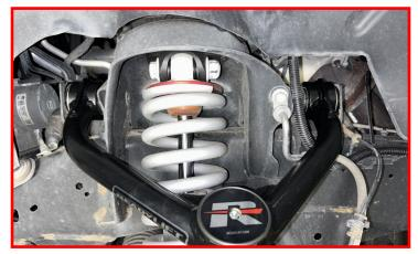
Torque the upper control arm hardware to 125 ft-lbs.
