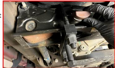
Push the torsion bar forward through the factory keyway cross member and lower control arm. You may need to use a hammer and punch on the end of the bar to break it loose from the keyway and control arm. Remove the torsion bar key.
