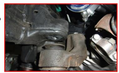
Install the 1/2" ReadyLIFT differential spacers between the frame and differential cradle. Use the provided laser cut washers and M14x130 bolts, reuse factory flange nuts.
