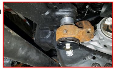
Install the differential skid plate with the rear mount only at this time. Insert the 1/2" spacers between the crossmember and skid plate. Use the supplied M10x40mm bolts and M10 fender washers.
