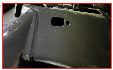
Press the fender liner towards the new hole and drill a 1/4" hole in the liner.
