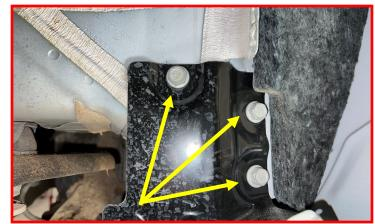
Remove the u-nuts from the black bracket and install them on the new fender bracket.
