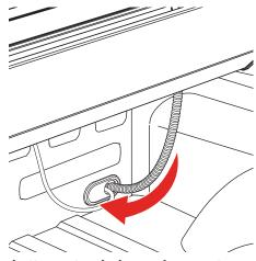
NOTE: For better water drainage, be sure to route the drain hose out of the truck in the most direct line as possible.
