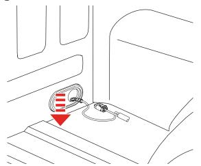
NOTE: If there is not a suitable hole in the bed, one may be drilled, but take great caution to be aware of lines and anything else behind where the hole is drilled. Keep the wires away from moving parts and exhaust.
