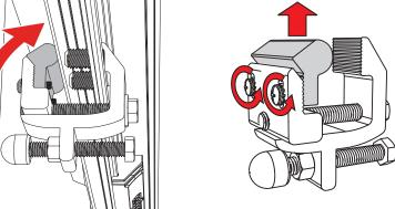
Insert a rubber shim (O) between the truck plastic bed cap and the truck metal rail at each clamping location behind the adjustment screws as shown below.
