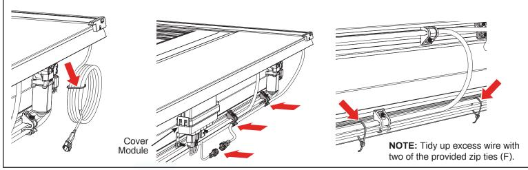
Before routing the main wiring harness (E) from the bed to the battery, first locate your battery in the engine compartment. Determine which side of the vehicle the battery is on - passenger or driver side - and then route the main wiring harness on the same side as your battery. Feed the battery terminal connection end of the main wiring harness (E) into the available pickup bed hole. Bring the wire down between the bed and the cab.
