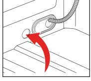
NOTE: Make sure to leave enough wire harness in the bed to attach to the cover module later in Step 16.
