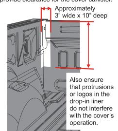
Position the cover: With two people, lift the cover and place it onto the truck bed starting by placing the canister (M) portion near the bulkhead. The front seal of the cover should lay forward and lay flat.
