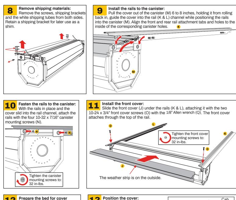
installation: NOTE: Prior to installing the cover, some drop-in style bed liners may need to be notched in the front/cab end corners to provide clearance for the cover canister.
