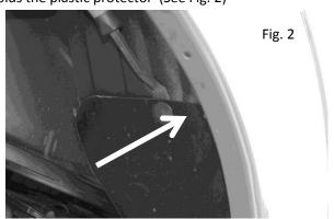
Insert the inner wheel well liner marked as (DS) under the inner panel of the wheel house.
