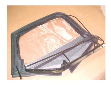
Pull bottom flaps up to meet Velcro. Now tighten the bottom Velcro to achieve the desired fabric-to-frame-to-retaining strip tension.
