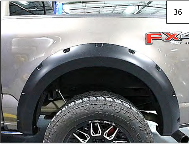
Completed Rear Flare Installation.
