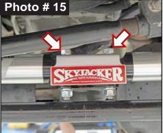
Washer & Nut. Tighten nut using a 11/16" socket\wrench until lock washer is compressed & bushing starts to swell slightly.
