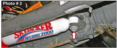
6. Cycle steering from side-to-side & check for adequate clearance. Check all brackets & bolts for proper installation.
