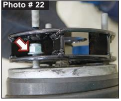
10mm Nylon Insert Flange Lock Nuts using a 15mm wrench. (Photo # 22) <u>Tech Note</u>: Start all three (3) OEM flange nuts before beginning tightening sequence. Torque 25 ft-lbs.
