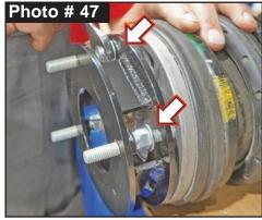
Attach Skyjacker Rear Strut Spacer on top of OEM strut assembly with supplied 10mm Nylon Insert Flange Lock Nuts using a 15mm wrench. (Photo # 47) **Tech Note:** Start all three (3) OEM flange nuts before beginning tightening sequence. Torque 25 ft-lbs.
