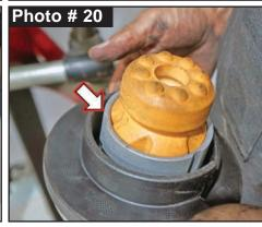
strut bump stop to upper rubber isolator & strut shaft. (Photo # 20)
