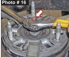
nut using a 18mm socket\wrench. (Photo # 16) Leave coil spring in spring compressor.
