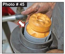
13. Align OEM top hat upper strut mounting isolator, rubber isolator & coil spring with previous marks & assemble Skyjacker\OEM strut assembly with OEM nut using a 18mm socket\wrench. (Photo # 40) Note: Make sure that your 'marks' align & that components are seated correctly into strut assembly alignment spiral.
